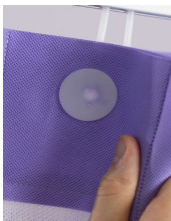
Robust hooks are ultrasonically welded.
